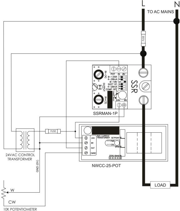
10K POTENTIOMETER SETS AC CURRENT VALUE AC CURRENT IS REGULATED AGAINST CHANGES IN LOAD OR LINE VOLTAGE
